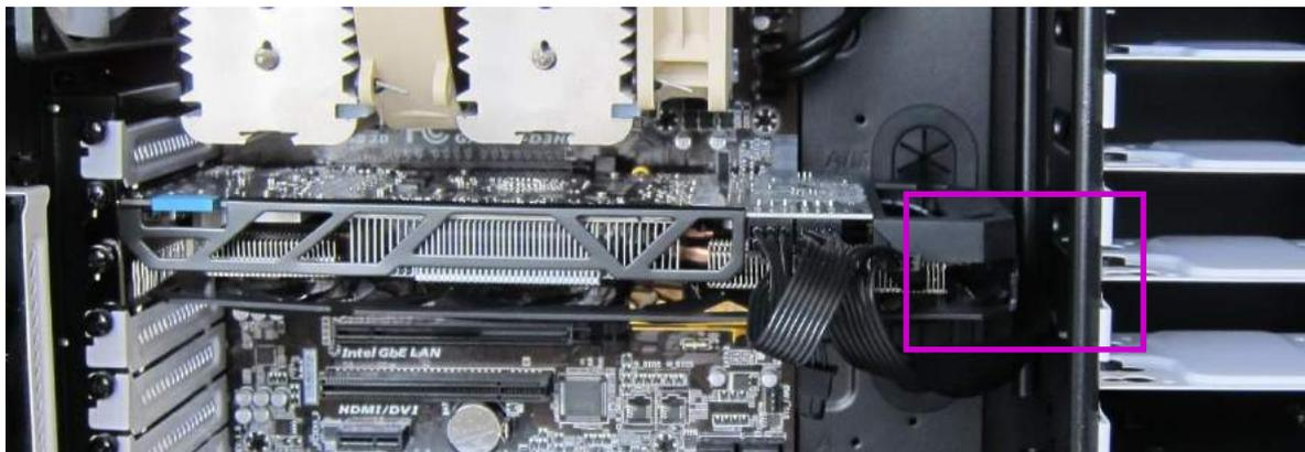
*Figure 12- A Graphics Card in case. A close fit, but this is compatible and fine for use.*
