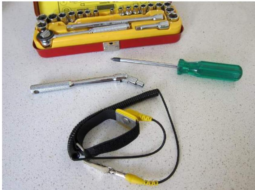
Figure 1 - A Philips head screwdriver, Anti-static wrist band and small socket set
