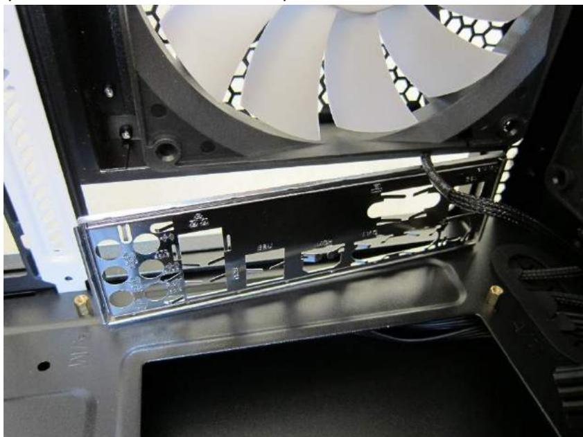
*Figure 4 - A motherboard backplate in a case*
