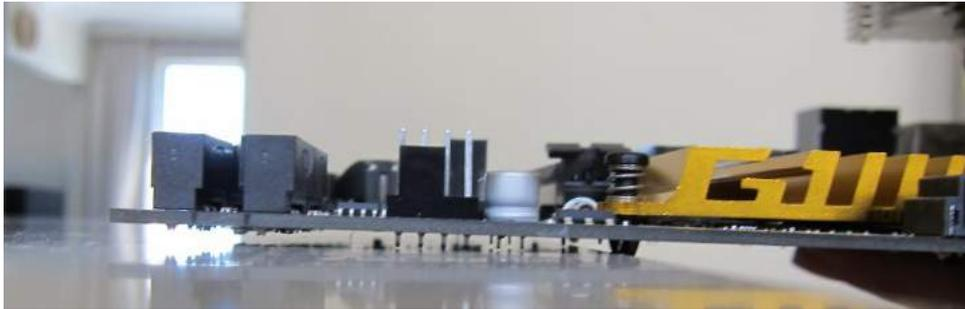
*Figure 16 - Where motherboard riser/standoffs are not used, the through hole pins sit directly on the grounded chassis - not good.*
