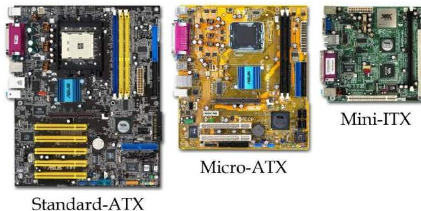
Figure 6 - Computer motherboard form factor types. Source: VIA Motherboards.
