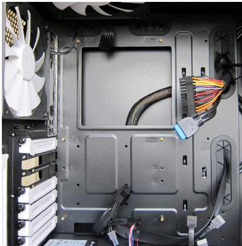
Figure 19 - Motherboard mounting points on an ATX motherboard (See 6 Gold coloured risers)
