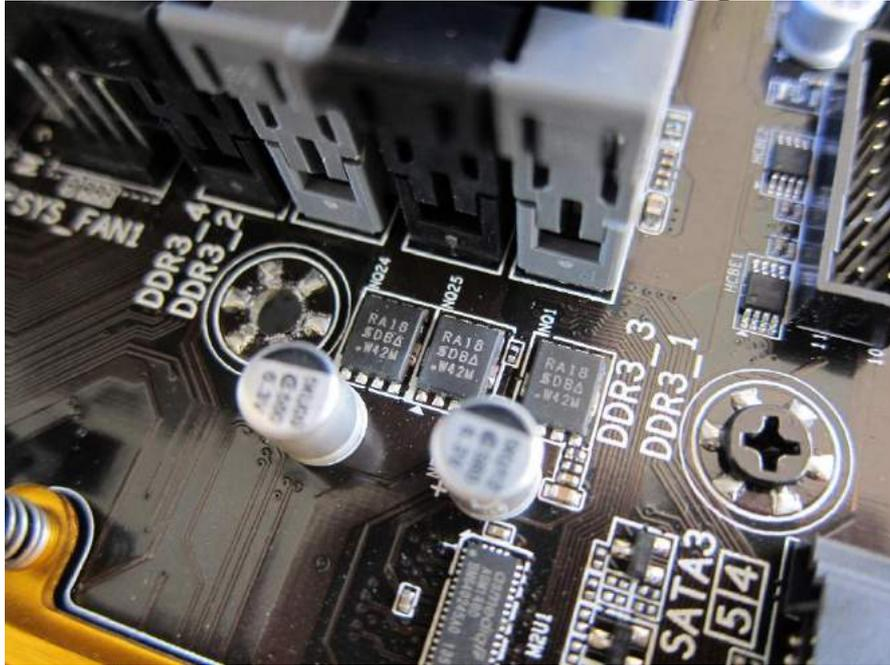
Figure 20 - A motherboard mounting point – LHS no mounting screw, RHS with mounting screw installed.
