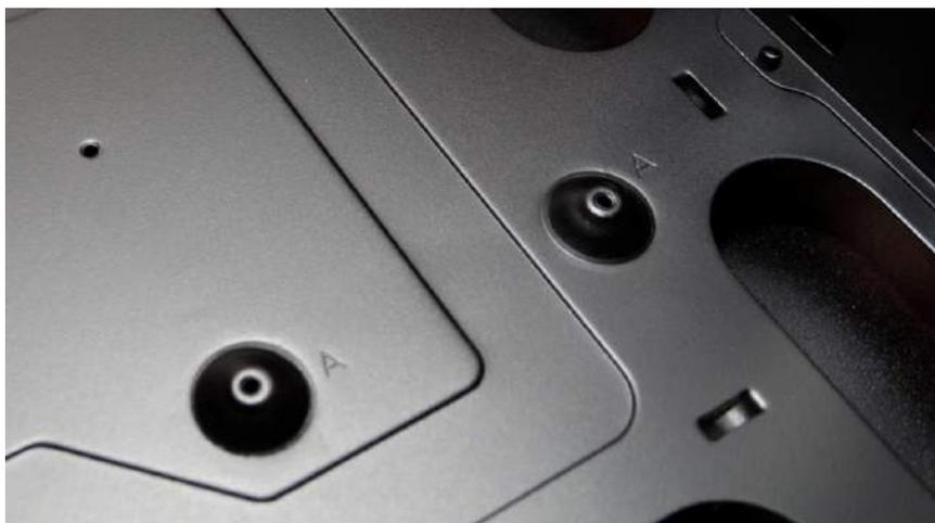
*Figure 17 - A case with inbuilt risers. Not always common, but handy.*
