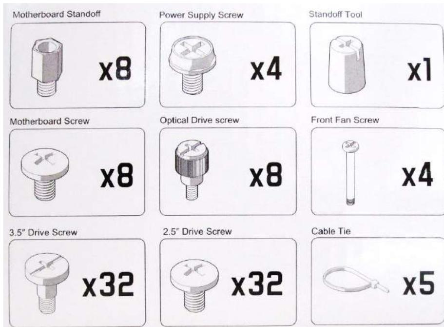
Figure 5 - A visual description of each of the screws which generally come with your computer case
