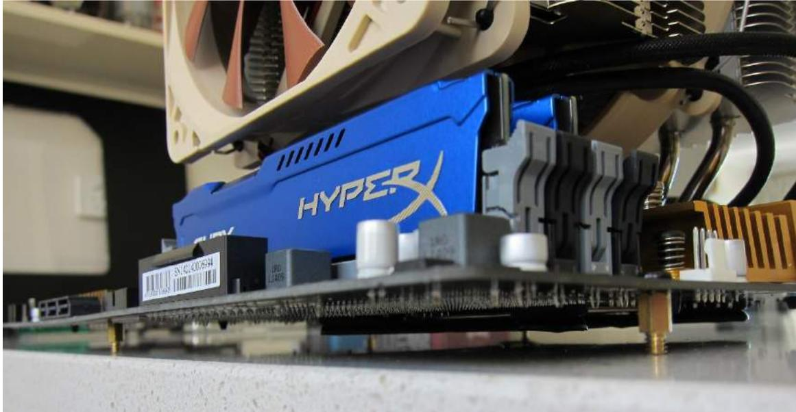
Figure 18 - The insulated air gap provided by risers / standoffs
