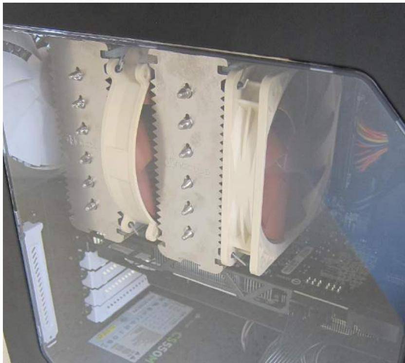
*Figure 13 - Aftermarket CPU cooler height - even a close fit in an ATX Mid Tower!*
