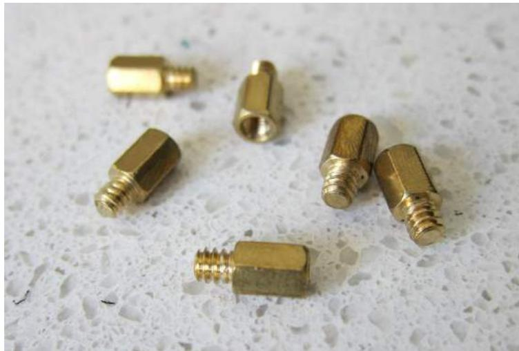
*Figure 14 - A motherboard riser / standoff*
